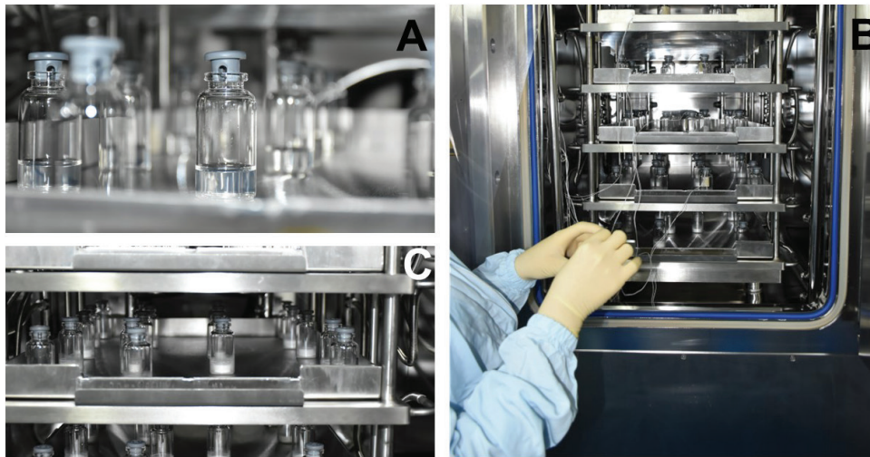
Figura 26. Lyophilization of antiophidic serum. (A) Antiophidic serum before lyophilization. (B) Antiophidic serum in lyophilization chamber. (C) Lyophilized antiophidic serum.
